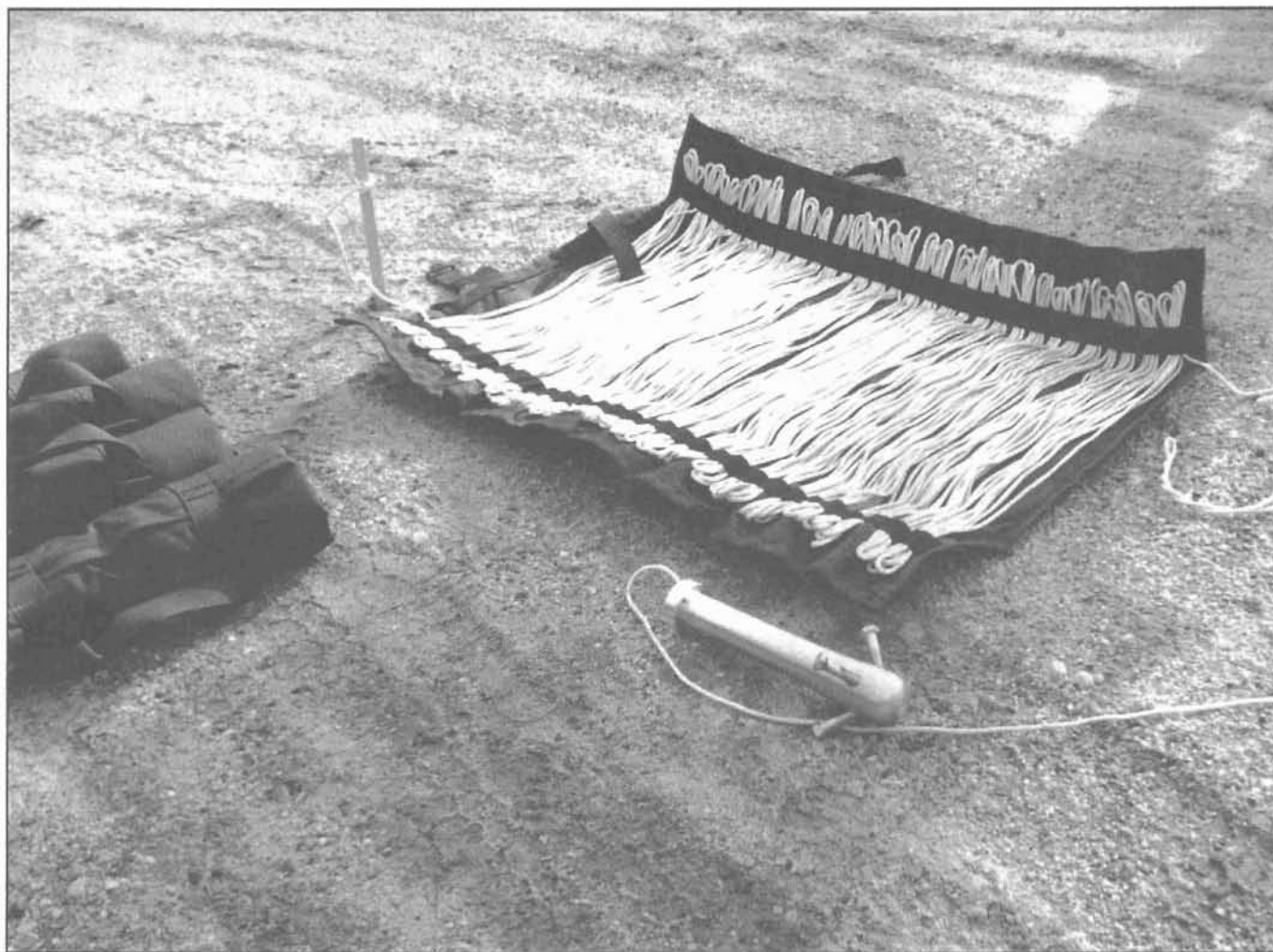
The bullet trap set, as tested at the National Training Center (NTC) and Fort Benning. Used by combat engineers in force-on-force exercises, the bullet trap proved easy to use and effective in clearing trip wires.
